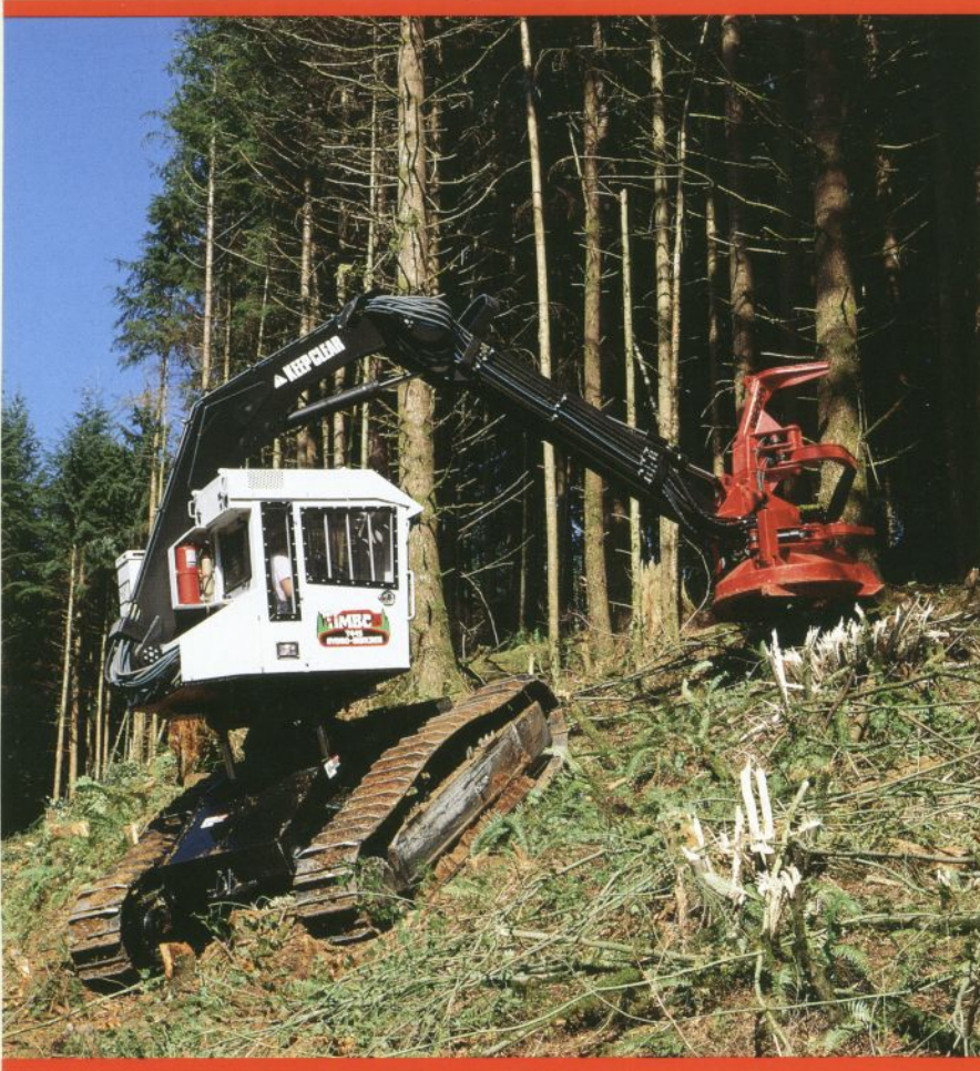
T445 shown with window bar protection, fire suppression, full halogen light package and 22" QUADCO™ disc saw attachment.
