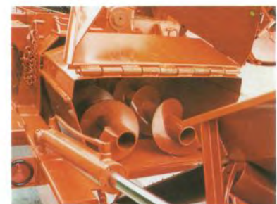
Less maintenance and more durable—the underneath dual auger discharge is far superior to a belt discharge.
