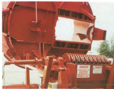
Hydraulic 90° tub tilt for quick clean out of material and debris and easy access to hammermill.
