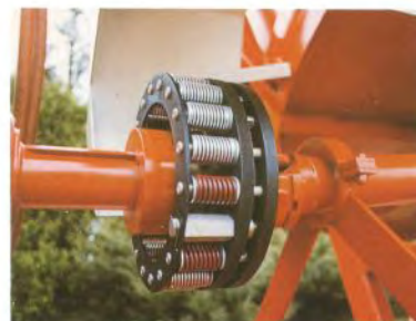
Torque limiter protects engine and clutch assembly against sudden shock or overload.
