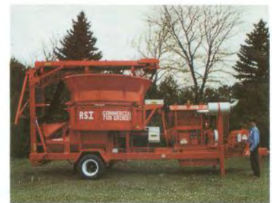
Discharge belt conveyor conveniently folds for transport.
