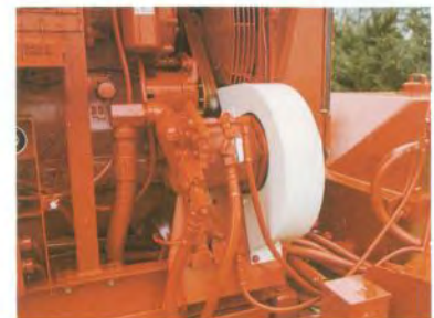
Pressure compensated hydraulic system means considerably longer pump life due to controlled oil flow and temperature.
